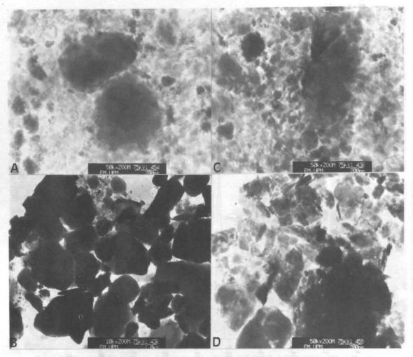
Plate 2: TEM micrographs of the clay fraction from the Ap (A) and Bt<sub>4</sub> (B) horizons of the soils at Kandy and from the A<sub>1</sub> (C) and Bt<sub>4</sub> (D) horizons of the soils at Anuradhapura
